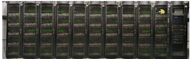
Fig. 1: The 1 million ARM-core SpiNNaker machine. Capable of simulating on the order of 200 million neurons, with 1,000 synapses each, in real-time.
